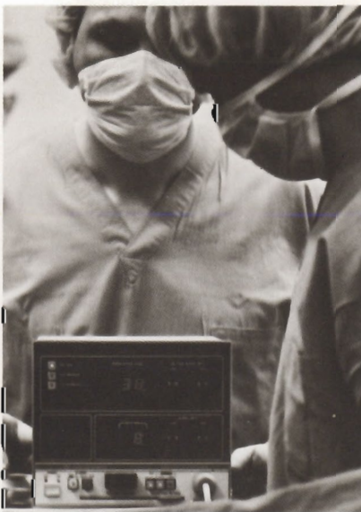
Medical team uses new HP capnometer (HP 47210A) to monitor patient's breathing.
